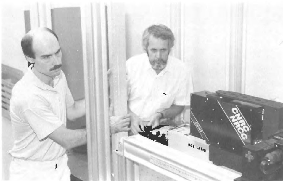
Luc Cournoyer (left) and Marc Rioux adjust and calibrate the NRC laser scanner using a cadmium/helium RGB laser for the simultaneous acquisition of both 3-D and colour data.
