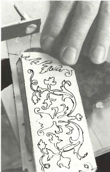
Cutting a replacement section through the "sandwich" of paper, tortoiseshell and brass.
