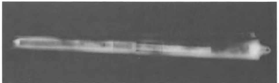
Radiograph of the whaling gun showing the lance stuck in the bore.
