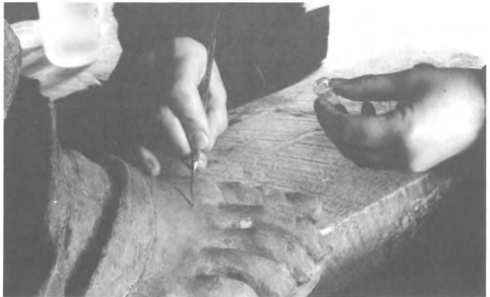
Figure 2. Taking samples of corrosion products from bronze for study and analysis.
