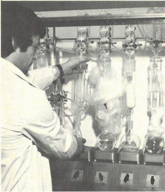
Chemical analysis for lignin and cellulose provides an indication of how badly degraded a piece of wood is. Here, a CCI scientist tests for the amount of lignin, which can remain in wood after years of burial, simply by removing the cellulose, easily hydrolyzed by acids, and weighing what is left.
