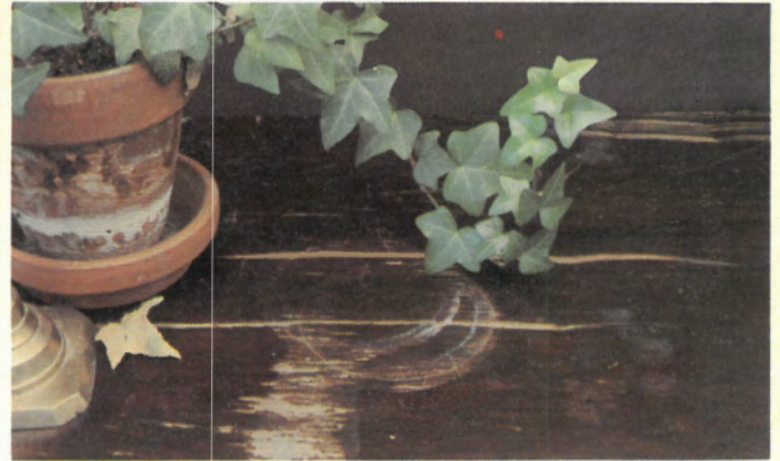
Plant pots placed on the top of this pump organ have caused the varnish to lift right off, ruining a once-attractive finish.
