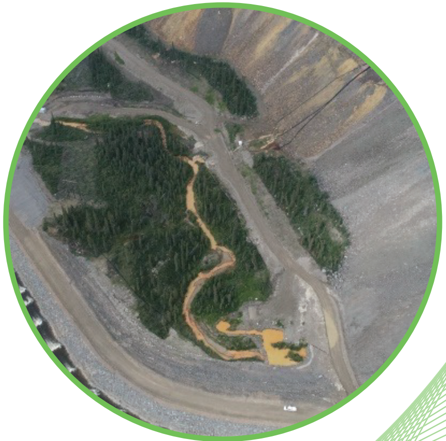
↓ Image: Contaminated water collection channel
