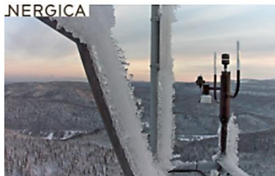
Figure 3.6: Ictek's IC-1 ice monitoring sensor [87].
