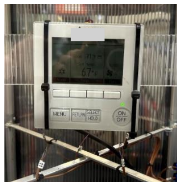
Figure 14. Unit C communicating thermostat in the thermostat environment emulator
