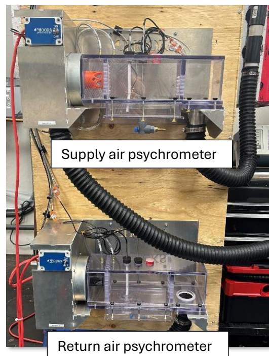
Figure 7. Supply and return psychrometers in the indoor test chamber
