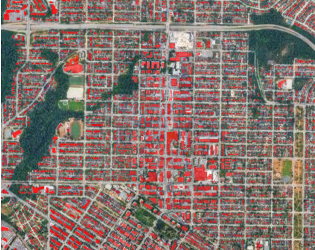
GeoAI for extracting foundational layers: North Vancouver, Automatically segmented buildings, 1967 and 2019.
