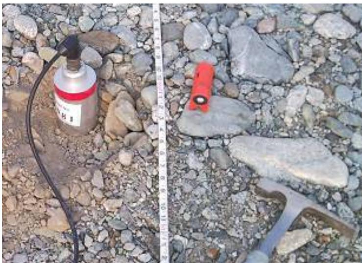
Figure 2.2.2-3. SASW receiver (1 Hz geophone).
