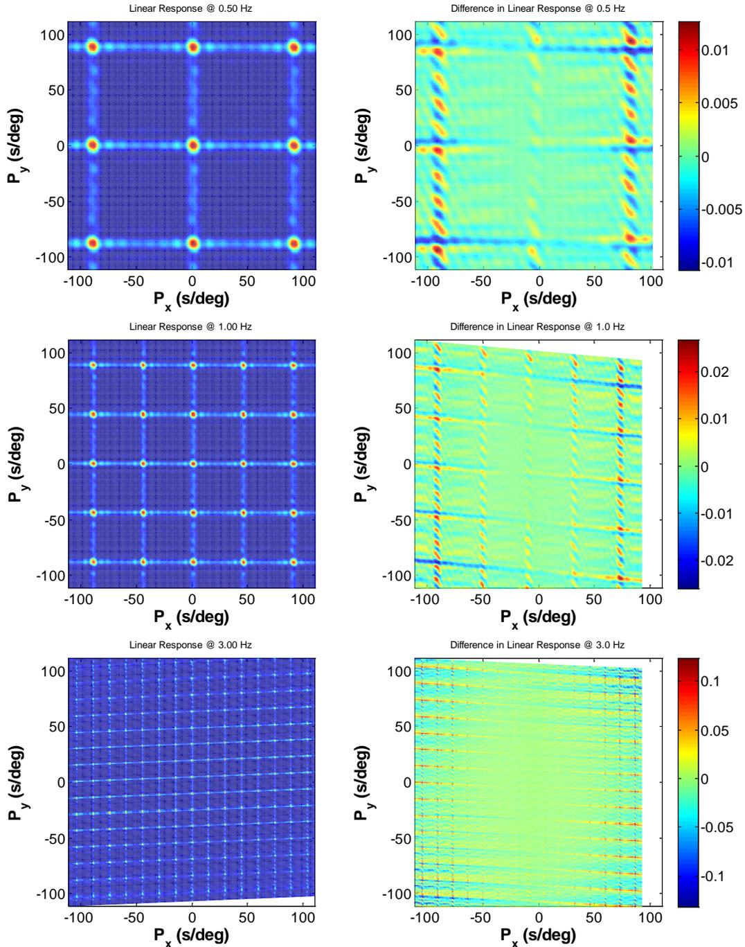
**Fig. 16:** Array responses for the new YKA at three frequencies (left) and the differences relative to its predecessor (right). Measurements are shown with a linear scale normalized to 1.0 at the response peak at  $(P_x, P_y)$  of  $(0, 0)$ . (Top) 0.5 Hz, (middle) 1.0 Hz, (bottom) 3.0 Hz. Residual magnitude scales are also linear, thus a 10% change in value would be represented as 0.1.
