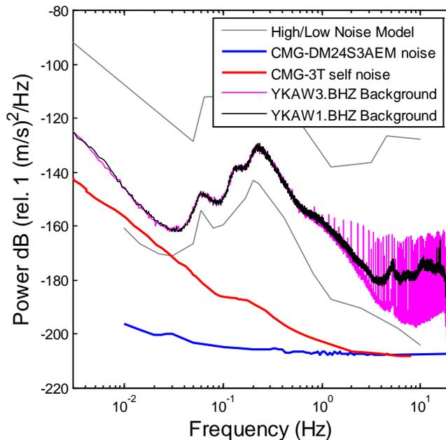
**Fig. 15:** Theoretical system noise for the new broadband stations at YKA. Both the measured CMG-DM24S3EAM digitizer noise using terminated input equivalent sensor impedance (blue line) and Guralp CMG-3T sensor self-noise as measured by Ringler and Hutt (2010) (red line) lie mostly below the low seismic noise model and typical low background levels for YKAW1 and YKAW3 (black/purple lines).
