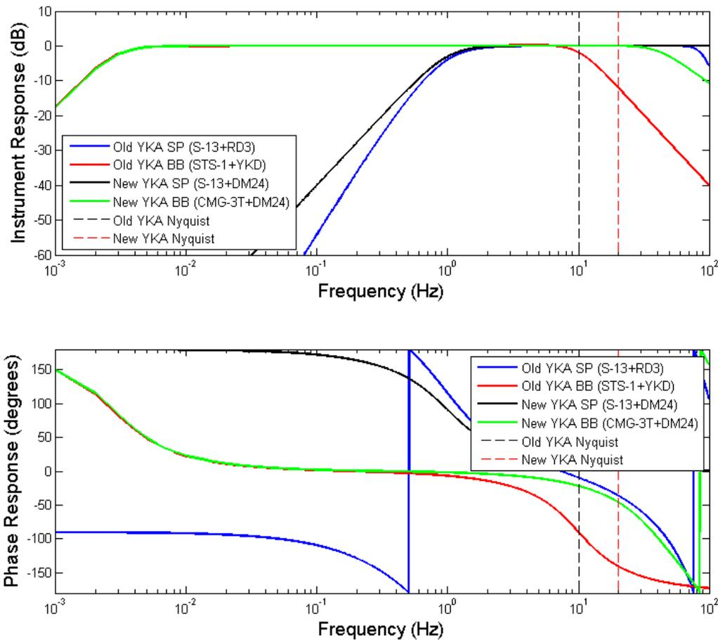
**Fig. 5:** Responses for the old Yellowknife short period (S-13/RD3 – blue) and broadband (STS-1/YKD – red) instruments versus the new Yellowknife short period (S-13/DM24 – black) and broadband (CMG-3T/DM24 – green) instruments.
