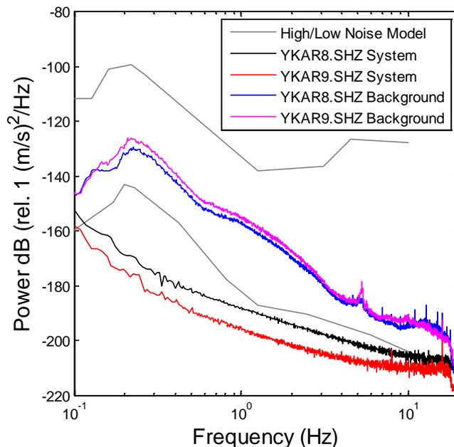
**Fig. 13:** System noise measurements at short period stations YKAR8 and R9 (red/black lines). Measured system noise sits below the Low Noise Model (Peterson, 1993), and indicates the limit to which a seismic event is discernible by YKA. Typical median low seismic background noise levels are shown for reference (blue/purple lines).
