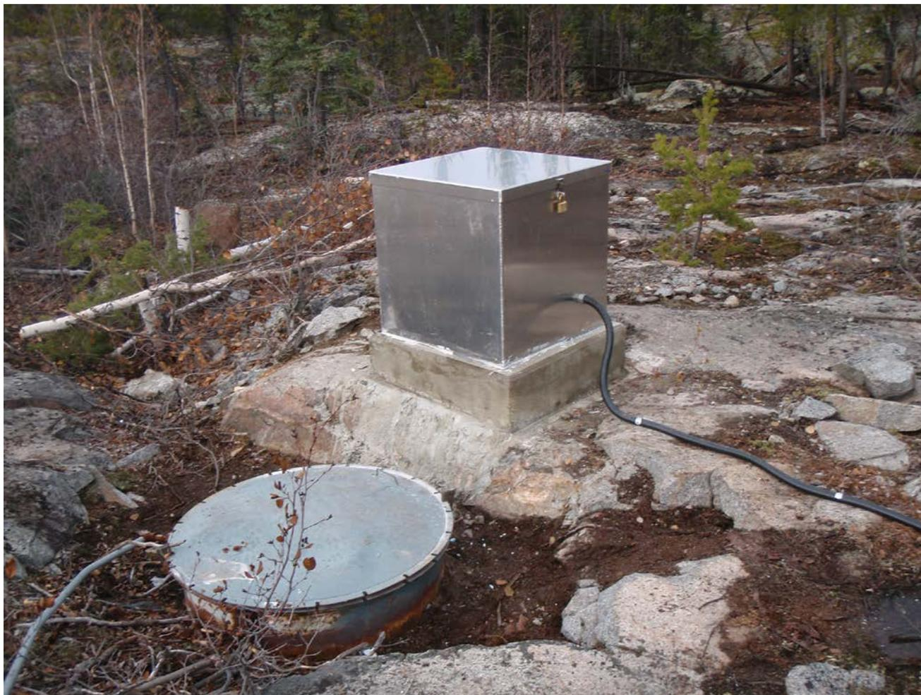
**Fig. 7:** Image of the old and new short period vaults at YKAB6. The original vault consisted of two welded half-cylinders blasted into the bedrock, fixed in place with a concrete base and sealed with a convex lid (left). The new vault (right) is a two-stage surface vault consisting of a concrete base, with a sealed inner HDPE vault and outer insulated aluminum vault.
