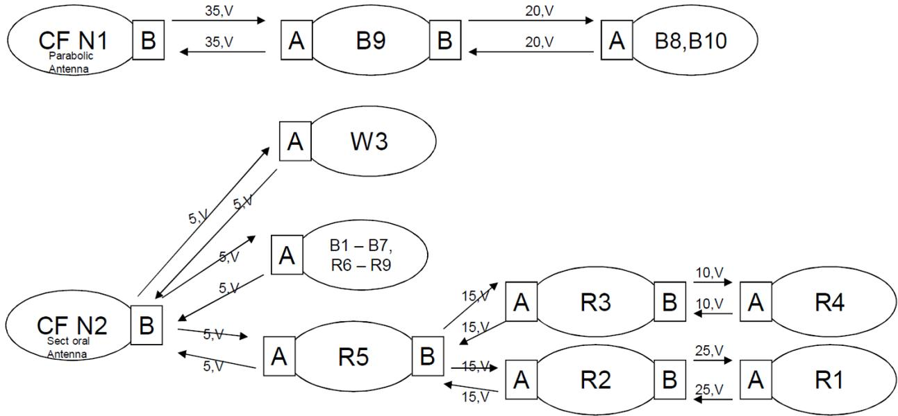
**Fig. 10:** Schematic diagram of the new Yellowknife seismic array Wi-LAN subnets to/from the Central facilities building.
