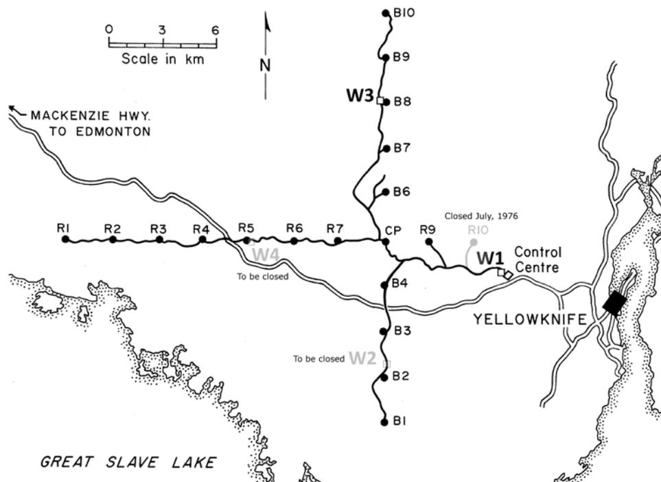
**Fig. 6:** Layout of the 2013 recapitalized Yellowknife seismic array. The complex consists of an eighteen (18) element short period array with two (2) broadband stations.
