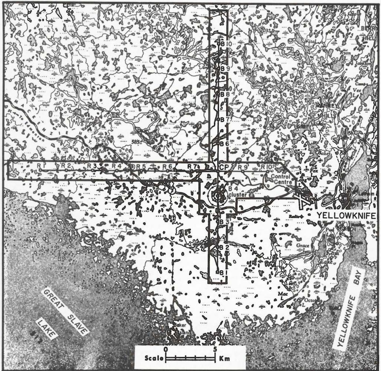
**Fig 1.** Layout and local property boundaries for the original Yellowknife seismic array (YKA). Station included 19 individual short period stations along two arms, spanning 25 km in length, and a small ~2 km aperture circular array. Reproduced from Manchee & Somers (1967).
