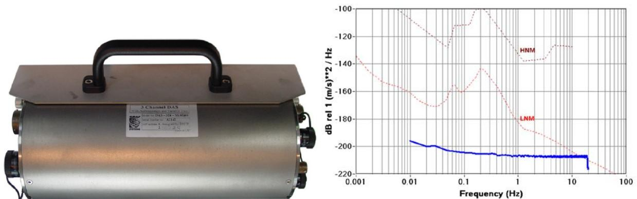
**Fig. 4:** The Guralp CMG-DM24S3EAM digitizer is the IMS preferred digitizer for the new YKA (left). This 24 bit digitizer replaces both the YKD and RD3 digitizers and includes onboard authentication and CD1.1 data output, required by all IMS stations. (right) Measured self-noise for the CMG-DM24S3EAM (gain setting of 2, using a reference sensitivity of 6000 V/(m/s)) is consistently below the seismic low noise background (Peterson, 1993).
