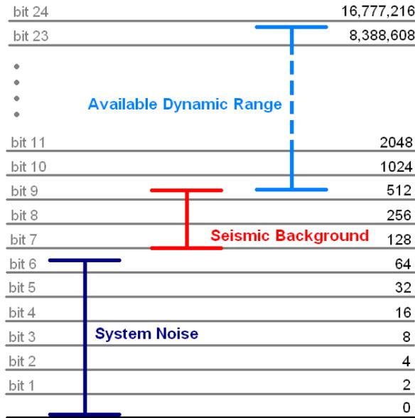
**Fig. 14:** Schematic diagram of the short period array use of available 24 bit dynamic range of the CMG-DM24S3EAM.
