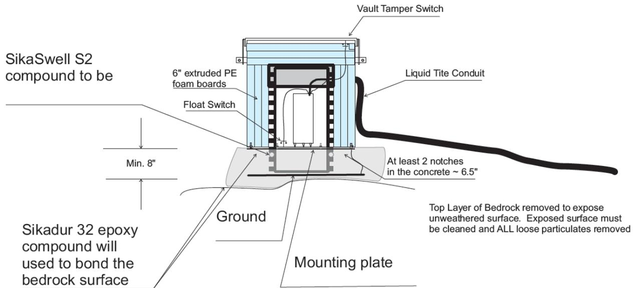
**Fig. 8:** Schematic diagram of the new Yellowknife short period vaults. The overall outer dimensions are 30” (76.2 cm) square, atop a minimum 8” (20.32cm) thick concrete slab. Inner vault is circular with a diameter of 37.5 cm.
