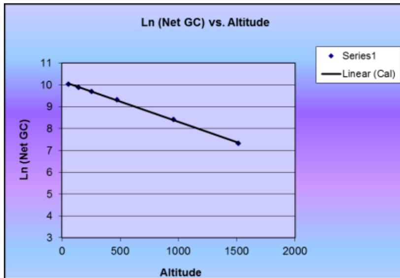
FIGURE 23 AMS RESULTS OF ALTITUDE SPIRAL OVER LAKE MOHAVE CALIBRATION RANGE. PLOTTED AS LOG OF NET GC.
