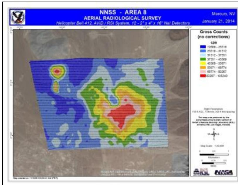
FIGURE 37 CONTOUR OF GROSS ACTIVITY FROM NNSS AREA 8 CREATED USING AMS DETECTION SYSTEM AND AMS DATA PROCESSING TECHNIQUES (2014-01-21 AM)
