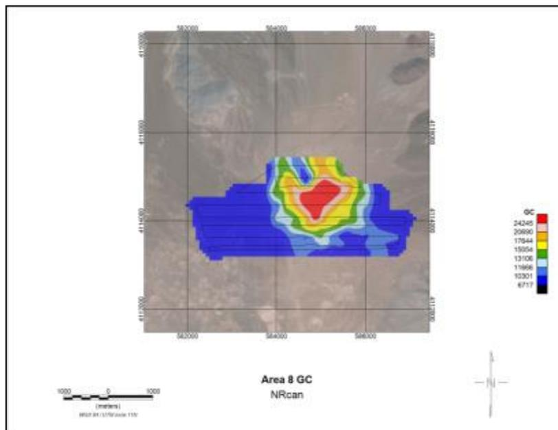
FIGURE 38 CONTOUR OF GROSS ACTIVITY FROM NNSS AREA 8 CREATED USING NRCAN DETECTION SYSTEM AND NRCAN DATA PROCESSING TECHNIQUES (2014-01-21 PM)
