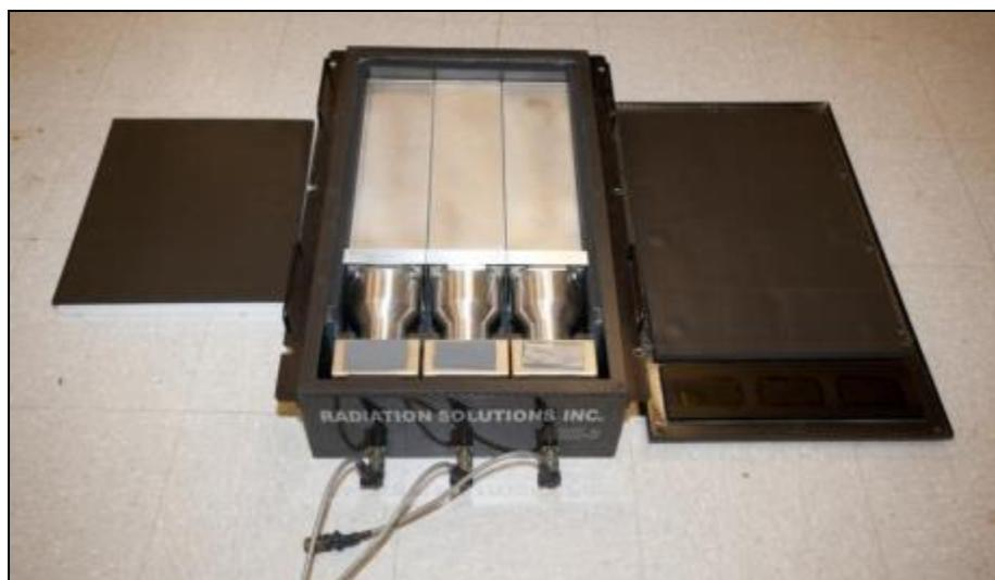
FIGURE 3 RSX-3 BOX WITH THREE 2" × 4" × 16" NAI(TL) CRYSTALS.
