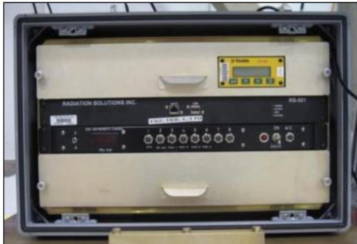
FIGURE 5 RS-501 AGGREGATOR CONSOLE WITH THE TRIMBLE GPS RECEIVER.
