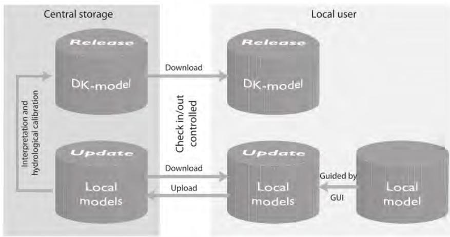
Figure 5. Workflow showing how local updates are pushed to central storage and eventually incorporated in to the Denmark regional model (from Højberg et al. (2013)).
