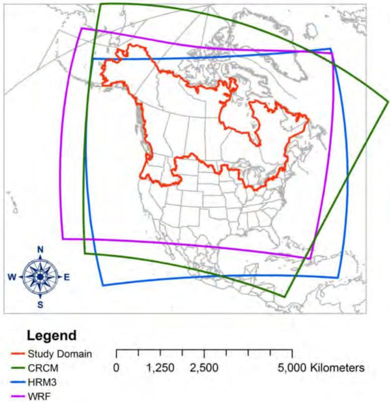
Figure 9. HydroGeoSphere model domain (red) and the regional climate model extents used to drive the HydroGeoSphere simulations (after Chen (2015)).
