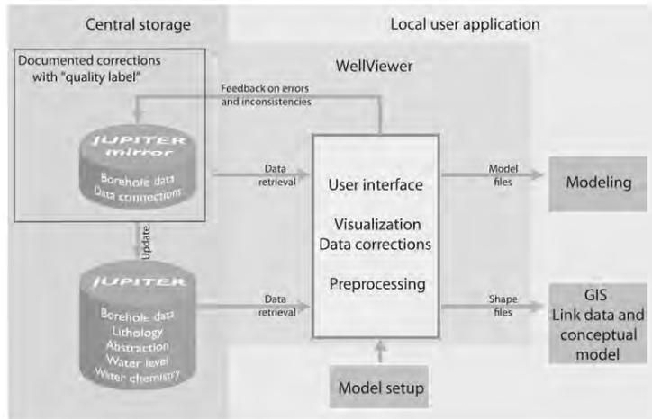
Figure 6. Framework for retrieving data from the central data, setting up a model, and pushing corrections/updates back to the central database (from Hojberg et al., (2013)).
