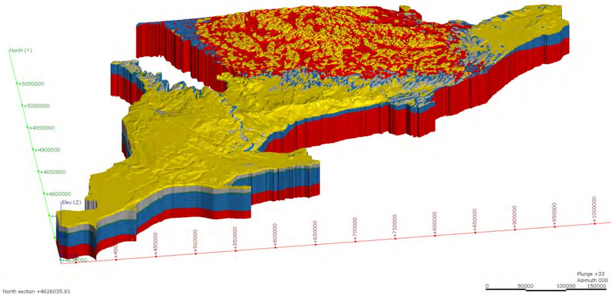
**Figure 25. Four layer geological model for Southern Ontario (from the Geological Survey of Canada).**
