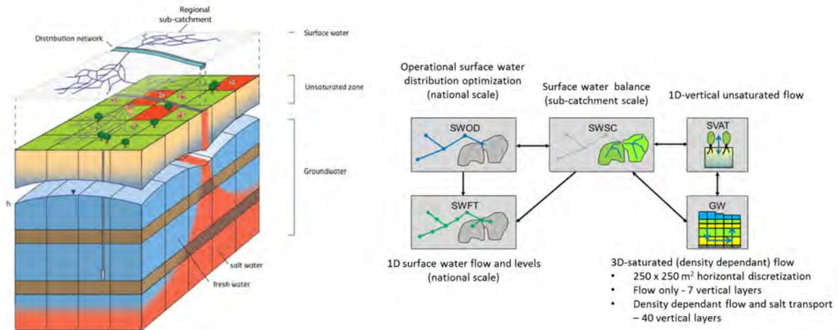
Figure 7. Schematic representation of the different hydrologic compartments considered within the Netherlands Hydrological Instrument and its five individual modelling components (modified from De Lange et al. (2014)).
