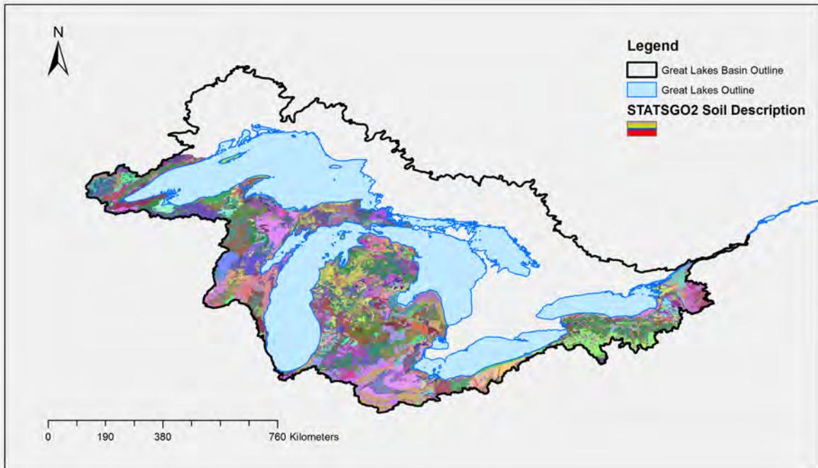
Figure 18. STATSGO2 soil class distribution for the U.S. portion of the GLB (STATSGO2).
