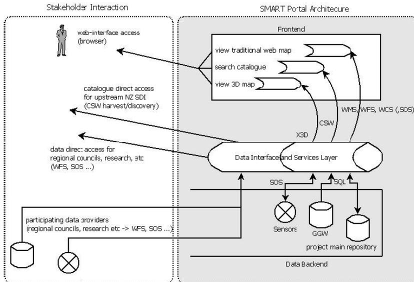
Figure 8. Conceptual architecture of the New Zealand SMART portal (after Knoch et al. (2012))
