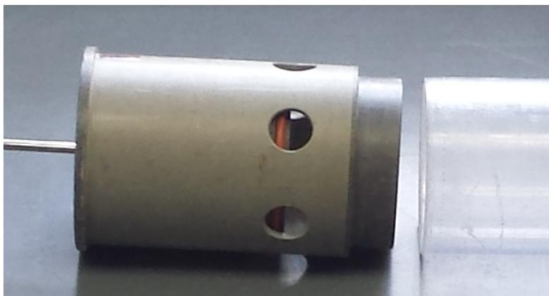
**Figure 6.** Auto valve on the head assembly of the Tech-Ops corer; Once the sediment seals the open end of the core tube, it creates a partial vacuum to prevent sediment from flowing out during ascent through the water column and retrieval. Photo: Geological Survey of Canada, May 2016
