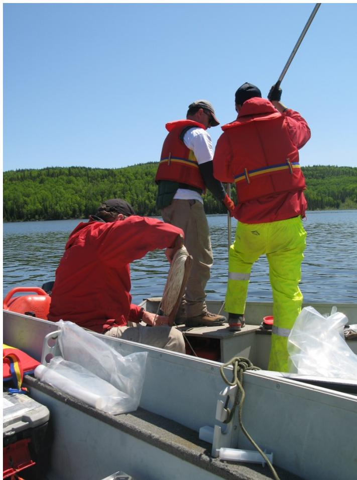
**Figure 8.** Attaching extension rod sections to the modified Tech-Ops gravity corer during its descent through the water column in Lac Dasserat; Photo: Geological Survey of Canada, May 2012
