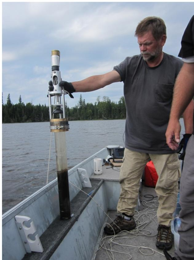
**Figure 2.** Deployment of the Glew corer in Lac Desvaux with insufficient core retrieval (< 30 cm); Photo: Geological Survey of Canada, July 2011
