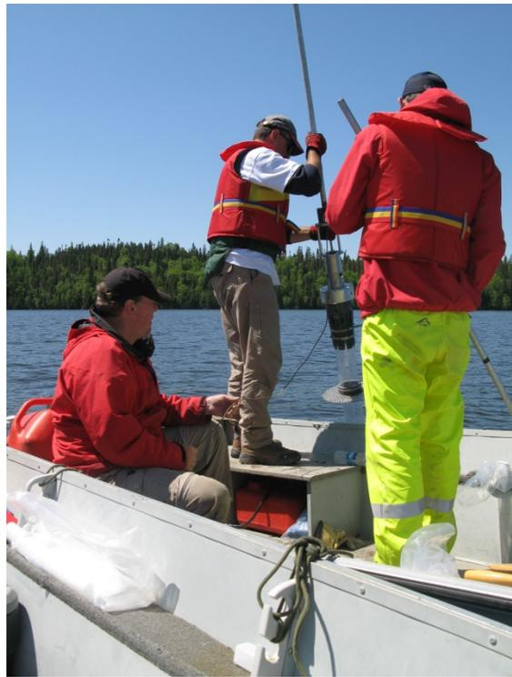
**Figure 15.** Routine operation of the modified Tech-Ops gravity corer; Photo: Geological Survey of Canada, May 2012
