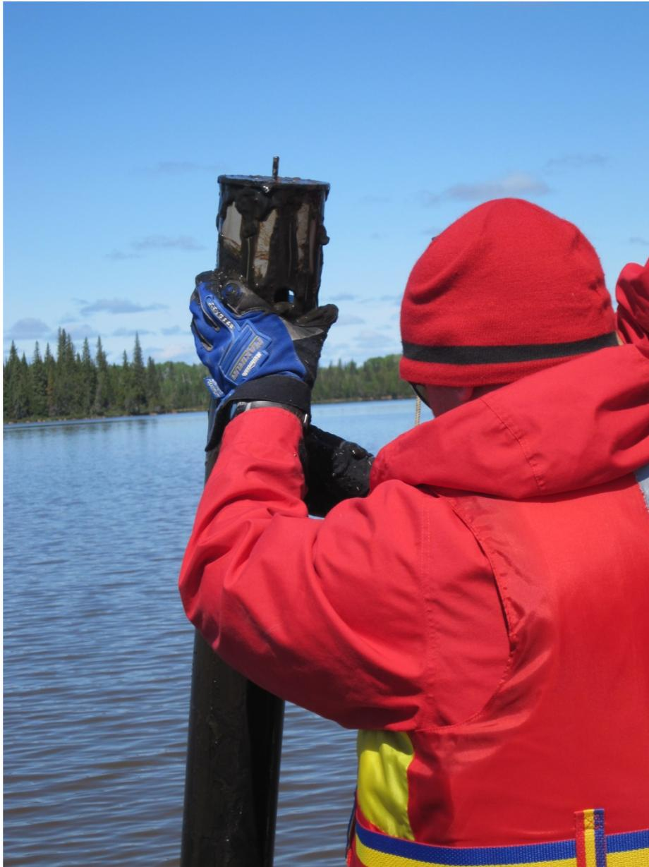
**Figure 12.** Sediment depth penetration was greater than the length of the core barrel, so that the sediments overflowed the top of the core barrel; the sediment-water interface was not preserved and the core discarded; Photo: Geological Survey of Canada, May 2012
