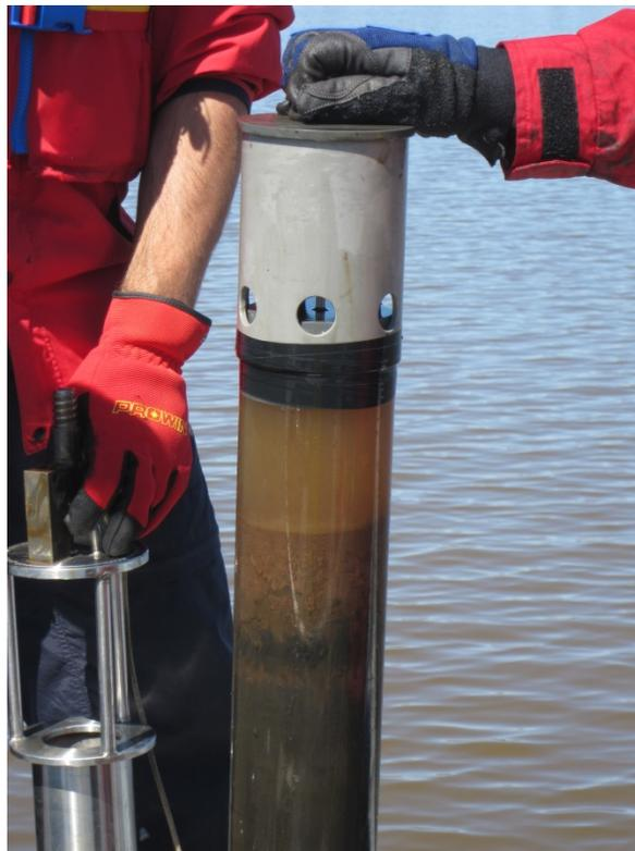
**Figure 14.** Preservation of the sediment-water interface and vertical distribution of chemical and mineralogical constituents from Lac Arnoux; Photo: Geological Survey of Canada, May 2012
