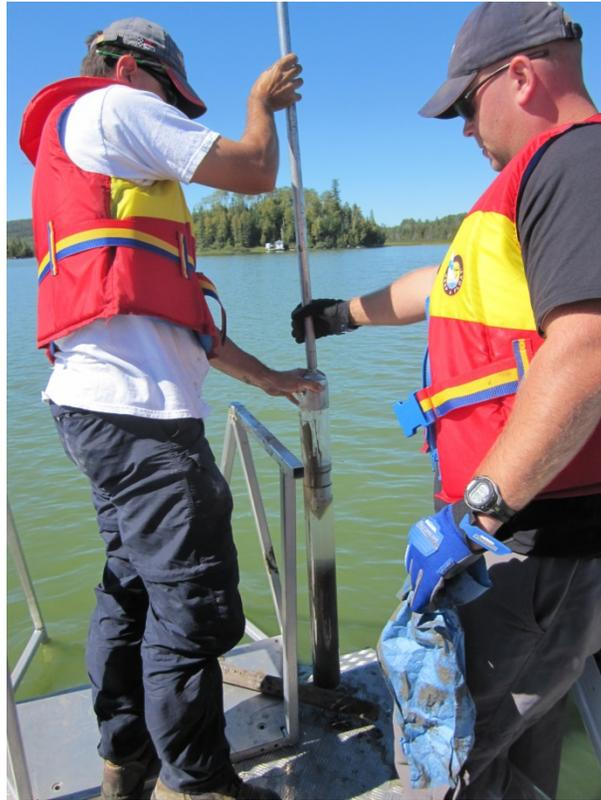
**Figure 3.** Test deployment of the Livingstone piston corer in Lac Desvaux; Photo: Geological Survey of Canada, Sept 2011
