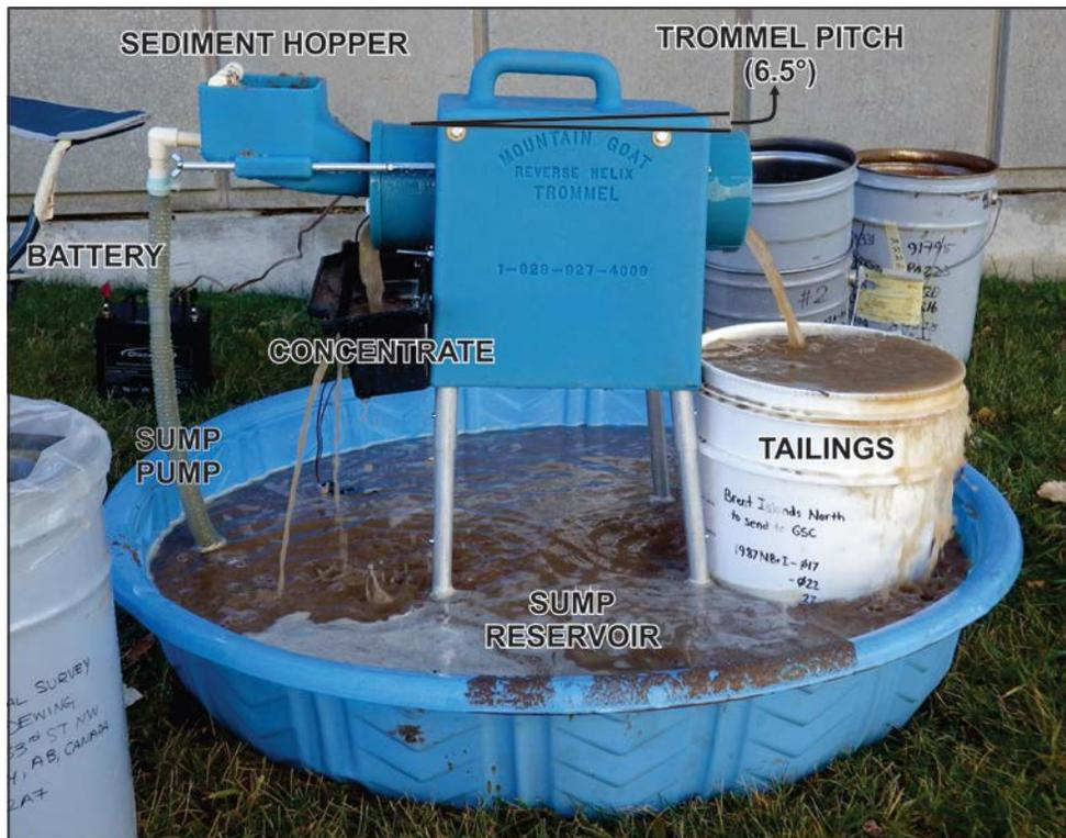
**Figure 3.** Mountain Goat Trommel spiral helix. Concentrated sediments are collected in the black pan at the back of the trommel, and then emptied into a separate sample bag.
