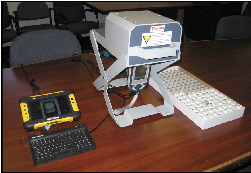
Figure 3: Example of XRF spectrometer mounted in a test stand with microcomputer for analysis of processed sediment samples. Photograph by R.D. Knight. NRCan photo 2020-926.
