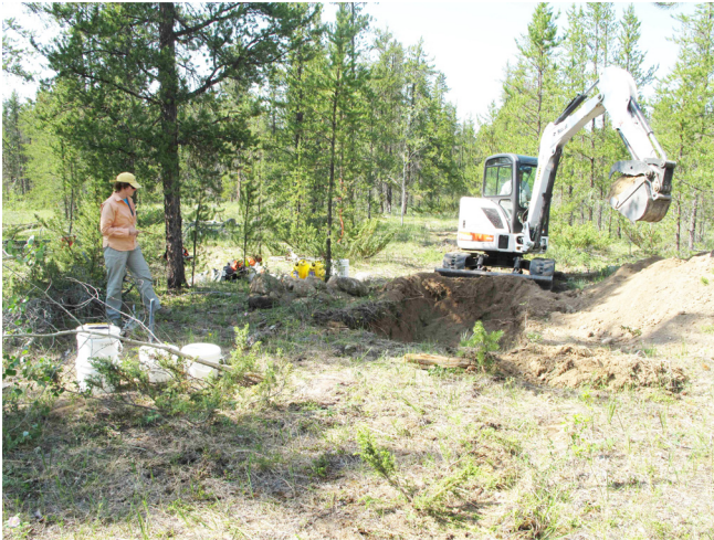
Figure 37. A small-tracked excavator used to dig trenches up to 3 m deep to collect till samples within and beneath highly oxidized surface till. Photograph courtesy of R. Paulen.
