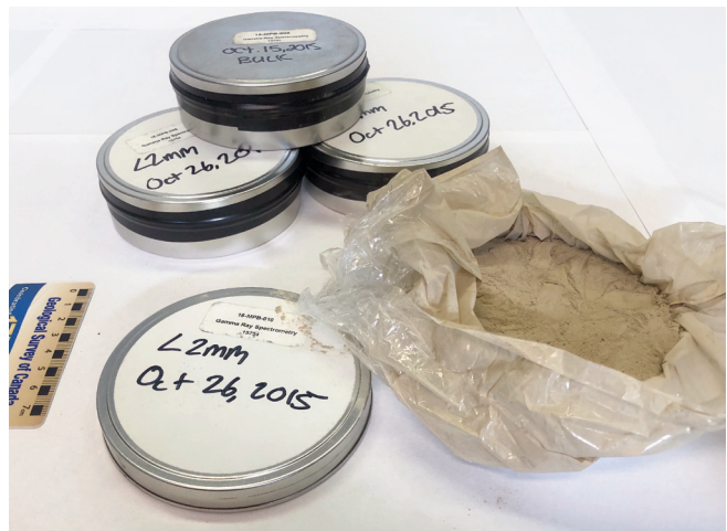
Figure 46. Photograph of metal tins filled with dried sieved till and sealed in preparation for gamma-ray spectrometry measurements to determine concentrations of the radioelements potassium (K), uranium (eU), and thorium (eTh). Photograph courtesy of B. McClenaghan.
