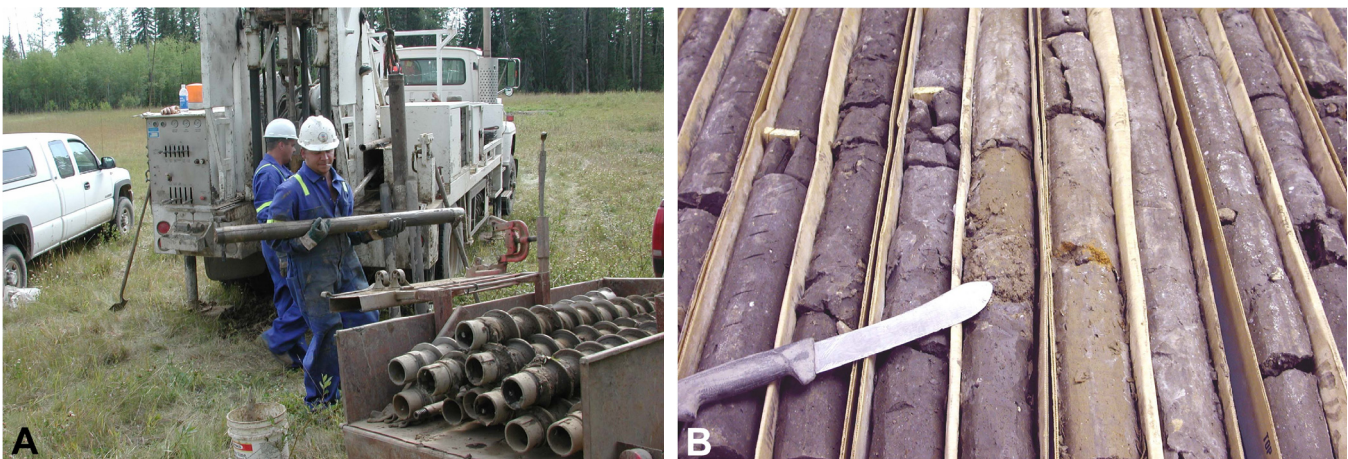
Figure 40. Photographs of a hollow-stem auger drill being used to recover till core for heavy mineral sampling in Alberta: a) removing the 1.5 m split core barrel, note the large 15.2 cm (6 inch) diameter hollow auger stems in the foreground; and b) an example of till core recovered by hollow-stem auger drilling (from Paulen, 2009).
