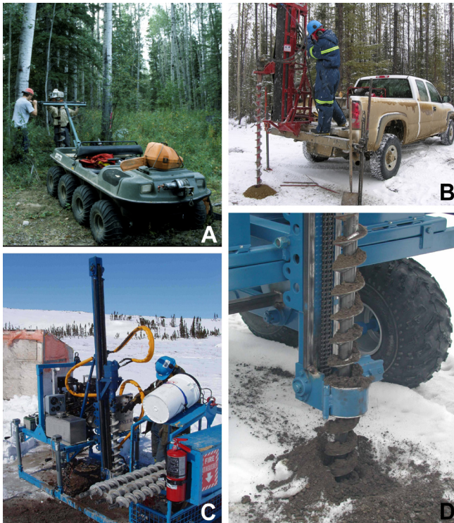
Figure 39. Photographs of solid-stem auger drills being used to recover till: a) a two-person auger with 15.2 cm (6 inch) diameter flights mounted on the back of an Argo® terrain vehicle to quickly obtain samples at 1 m depth; b) a Big Beaver® auger drill mounted on the back of a pick-up truck; c) a Pioneer® auger drill brought to a remote site in the Yukon by helicopter (photo courtesy of Multi-Power Products Ltd.); d) till recovered on 10.1 cm (4 inch) auger flights with a Pioneer® auger drill mounted on the back of an all-terrain vehicle (photo courtesy of Multi-Power Products Ltd.) (from Paulen, 2009).
