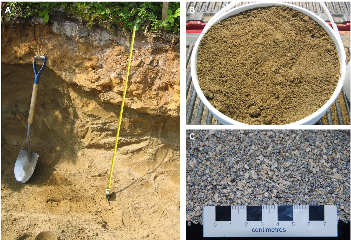
Figure 47. Photographs of GSC “Bathurst blank”: a) an unconsolidated weathered Silurian-Devonian granite (grus) collected near Bathurst, New Brunswick and used as the Geological Survey of Canada’s blank sand heavy mineral sample; b) the sample material in a 2.5 gallon bucket; and c) a close-up view of the blank sample material ( from Plouffe et al., 2014 ).
