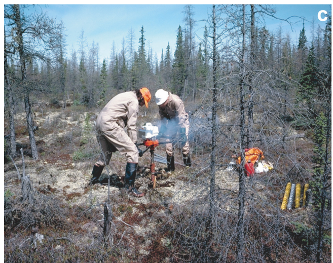
Figure 38. Photographs of portable drilling equipment: a ) a portable percussion drill used to collect till samples in Finland; b ) small (150–300 g) samples collected using the flow-through sampler on a portable percussion drill (photographs (a) and (b) from McMartin and McClenaghan, 2001); and c ) till sampling below thick peat using a semi-portable Sipre auger corer in northern Manitoba (from McMartin and Campbell, 2009).
