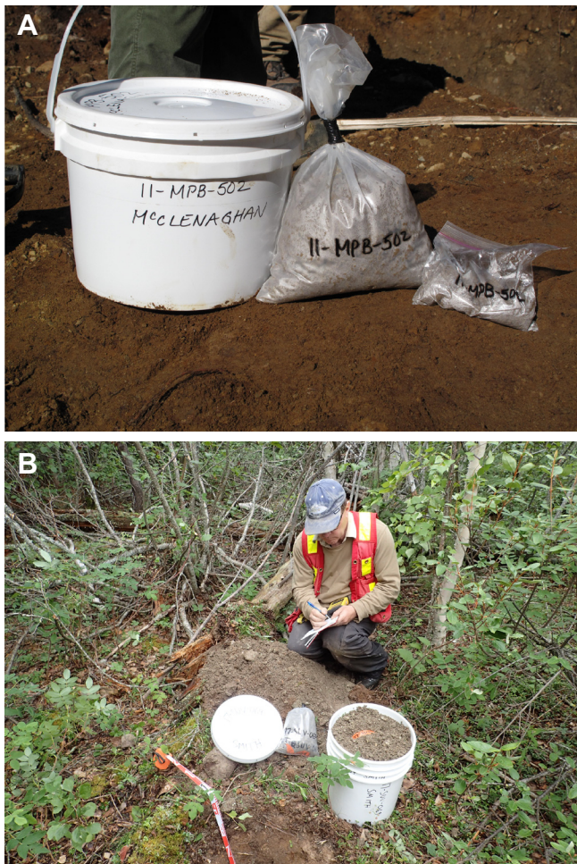
Figure 21. Photographs of (a) three samples of till that have been collected from the same site (a large 10–15 kg sample of sandy till for the recovery of heavy minerals; a 3 kg sample for matrix geochemical analyses, determining physical properties, and archiving; and a 300 g sample for pXRF analyses); and (b) a 20–30 kg sample of clay-rich till in a 19 L (5 gallon) pail lined with a plastic bag. Note that the sample number is recorded on both the pail and on a tag (flagging tape) inserted in the pail.
