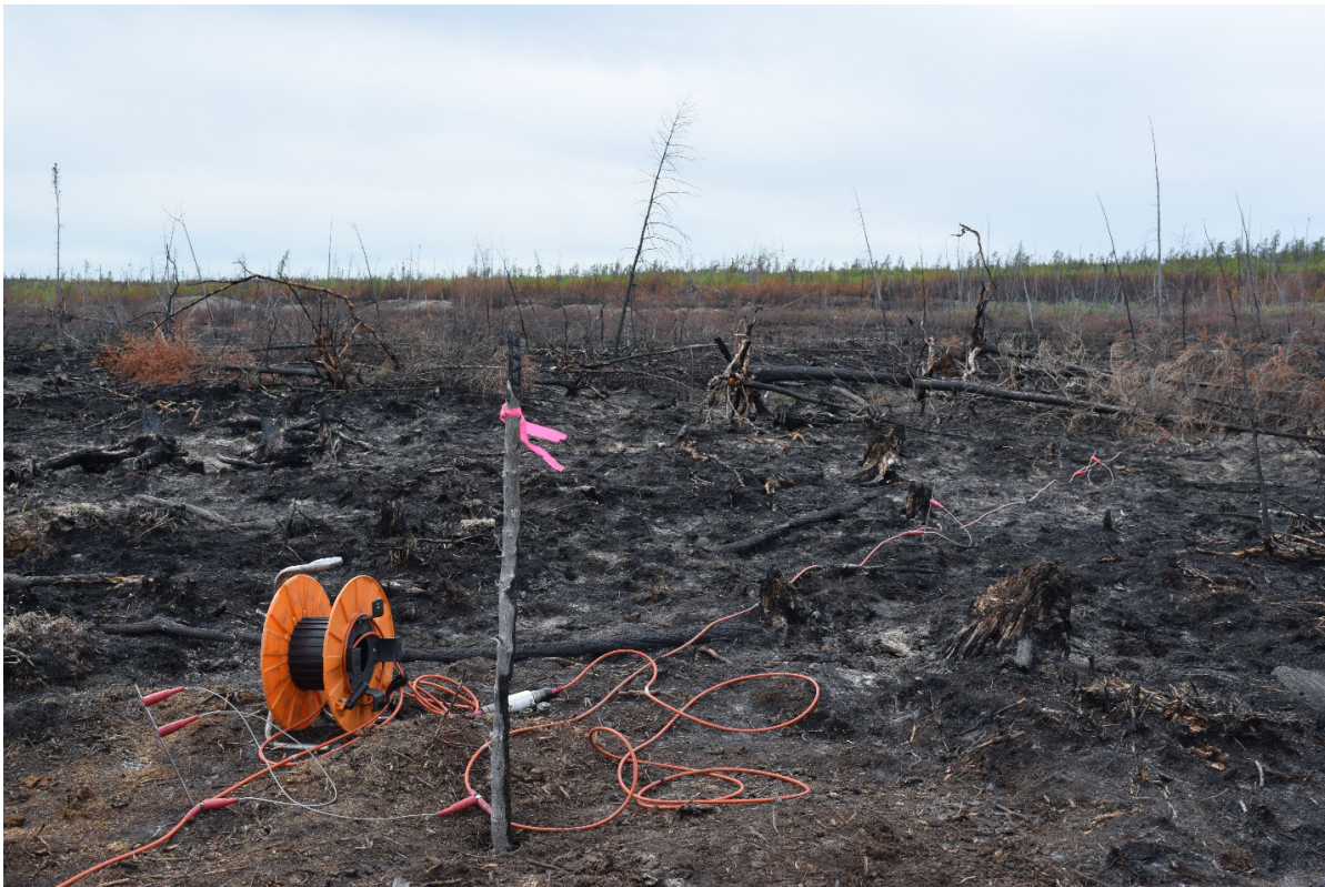
Figure 2. Electrodes and cables used in an electrical resistivity tomography survey conducted in August 2016.
