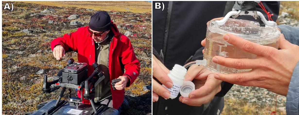
Figure 3: September 2023 field photographs of: A) UAV pilot É. Girard preparing a DJI Matrice 300 RTK Unmanned Aerial Vehicle (UAV), drone for planned aerial water sampling missions near Rankin Inlet, Nunavut; and B) collection of water samples from a Speedip device, ensuring transfer into well-sealed HDPE or glass bottles for subsequent geochemical analysis.
