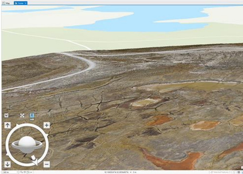
Reconstruction in 3D from drone images where ice wedge polygons are visible (black line in the left side of image) north of Rankin Inlet, Nvt.
