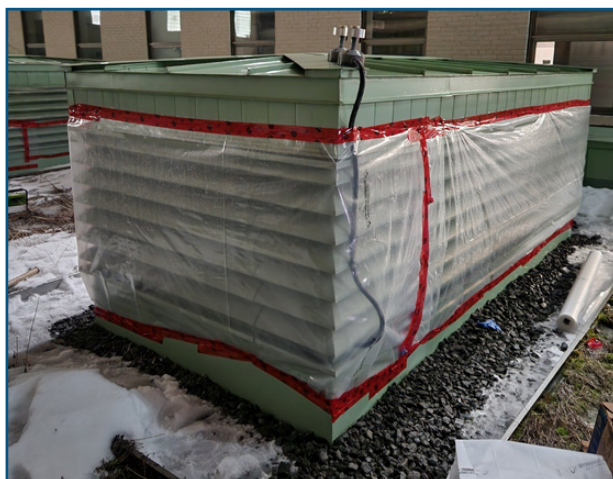
Figure 10: Configuration of envelope testing with sealed ventilation
