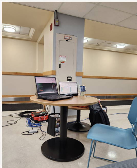
Figure 18: Wired network for airtightness testing connected to a laptop
