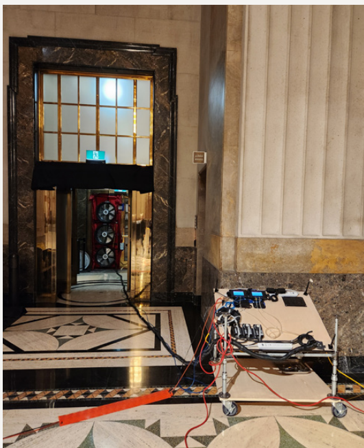
Figure 17: Wired network for airtightness testing
