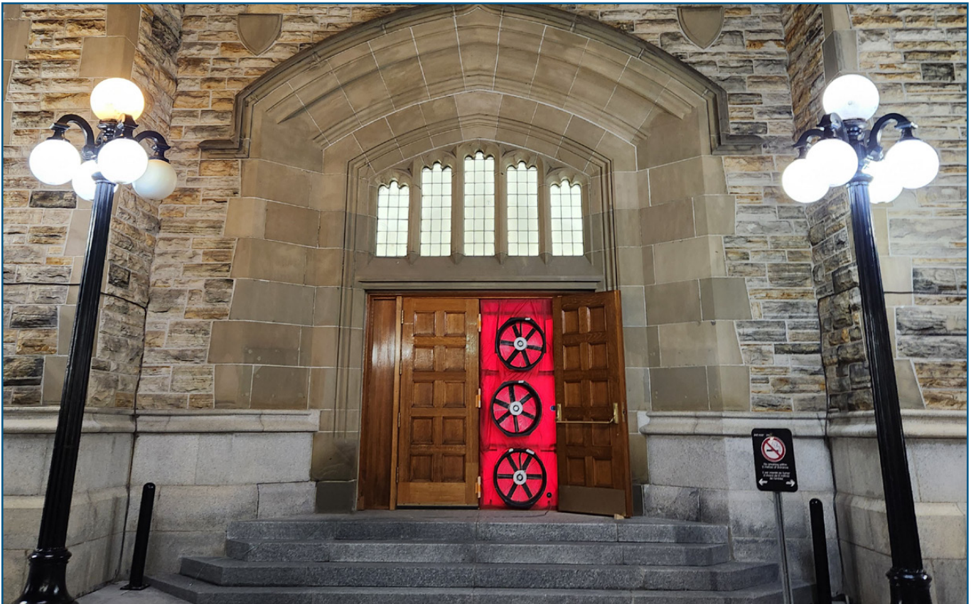
Figure 8: Blower door assembly for pressurization and depressurization
