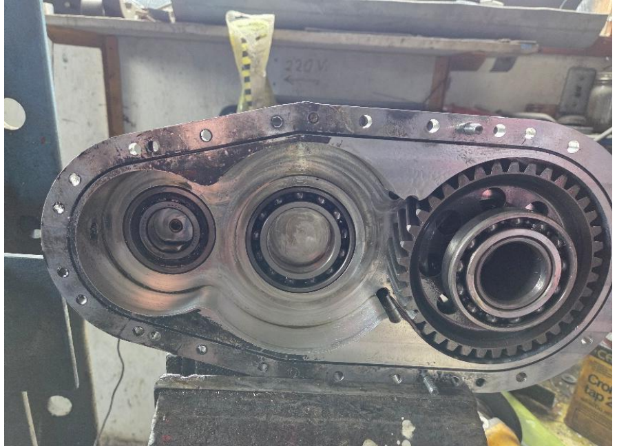
Image 1: Gearbox opened for inspection
