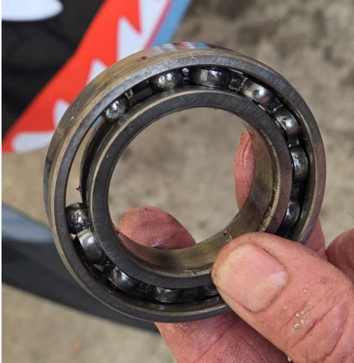
Image 3: Failed roller bearing
