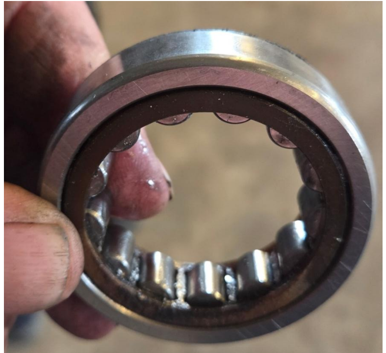
Image 4: Metal (silver) filings on another gearbox bearing
