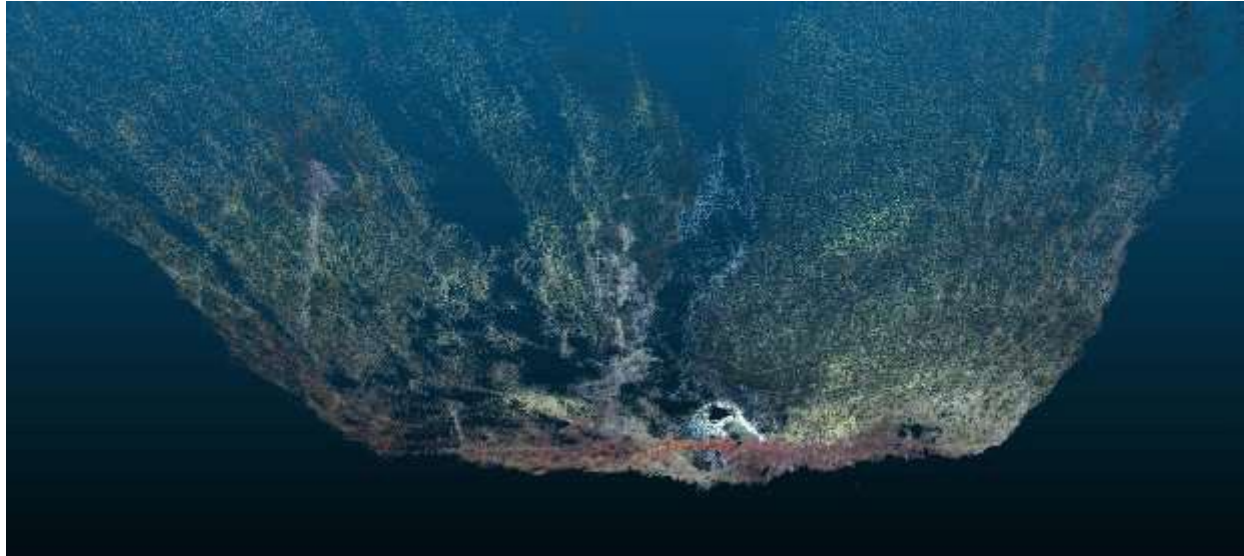
Figure 24. SfM 3D map generated based of 2D RGB images of the same scene (see Figure 23).
