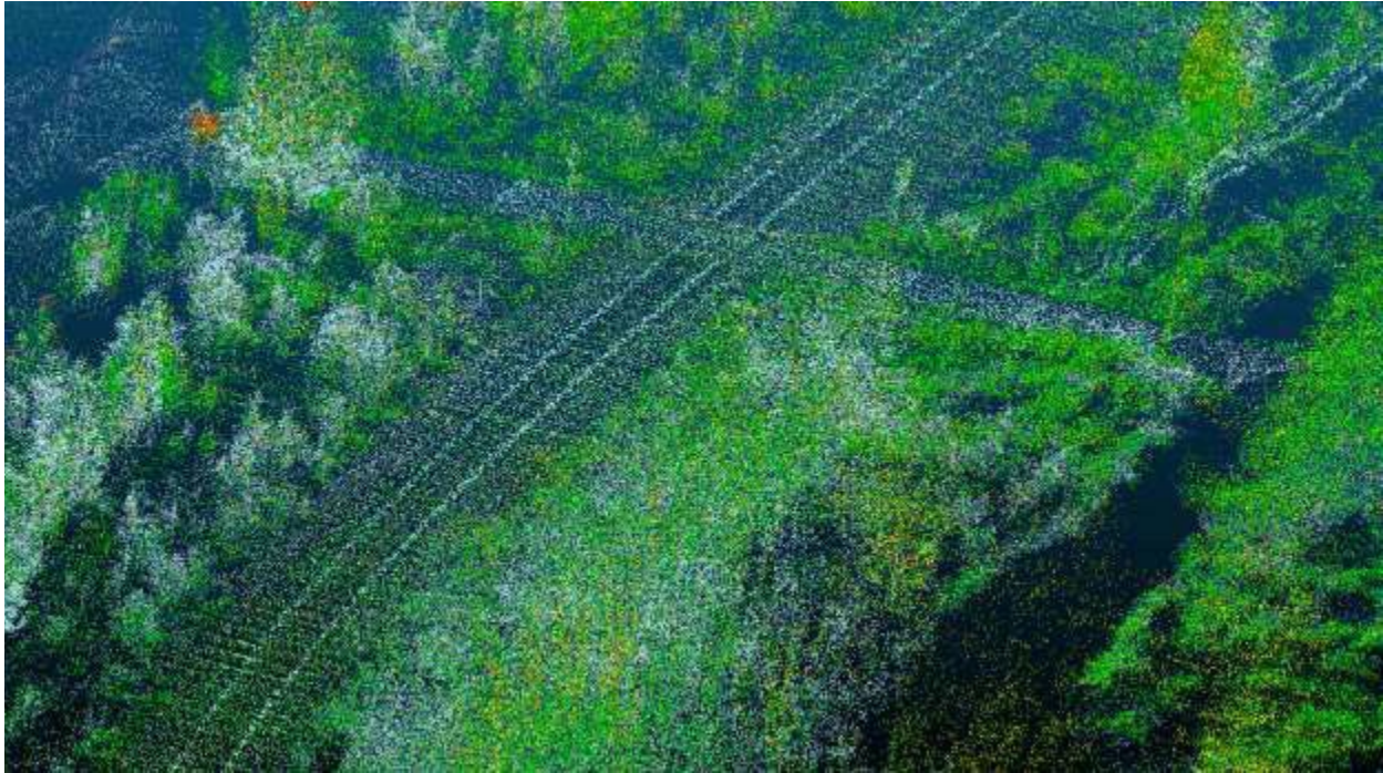
Figure 15. 3D point cloud map showing a railway track, a farm crossing, and the surrounding area.
