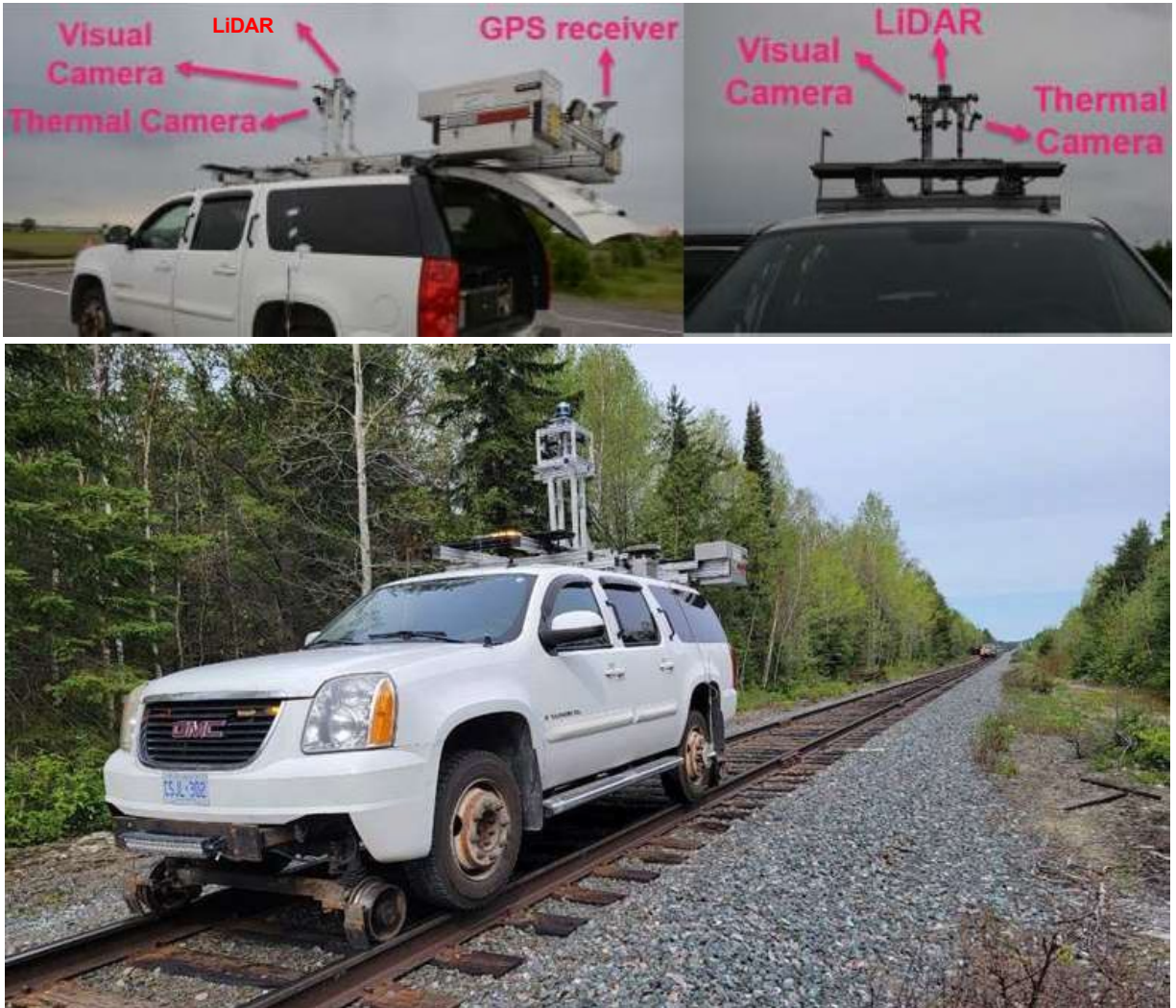
Figure 9. Instrumented hi-rail truck.
