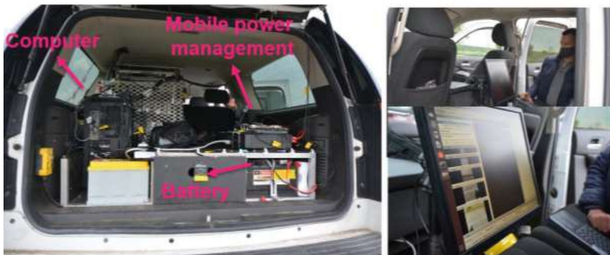
Figure 10. Auxiliary components for the DAQ (left) and in-vehicle visualization (right).
